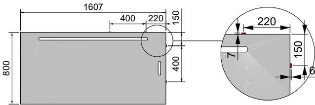
The magnets **protrude 7 mm** from the structure and are **offset** from the beam to which they are attached so that magnets from different desks do not conflict when joining 2 or more desks.
