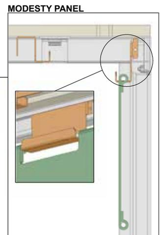
By inserting the **iron rods** into the appropriate **slots**, the fabric can be **hooked on both sides**, thus becoming a **cable holder**, as it is positioned exactly **under the long milling** of the desk.
